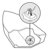
Inside the hull installations require no holes be drilled into the boat and through experimentation, highspeed operation comparable to transom mounting can be achieved. Two part, slow cure epoxy (not included) is required to glue the transducer in place.
